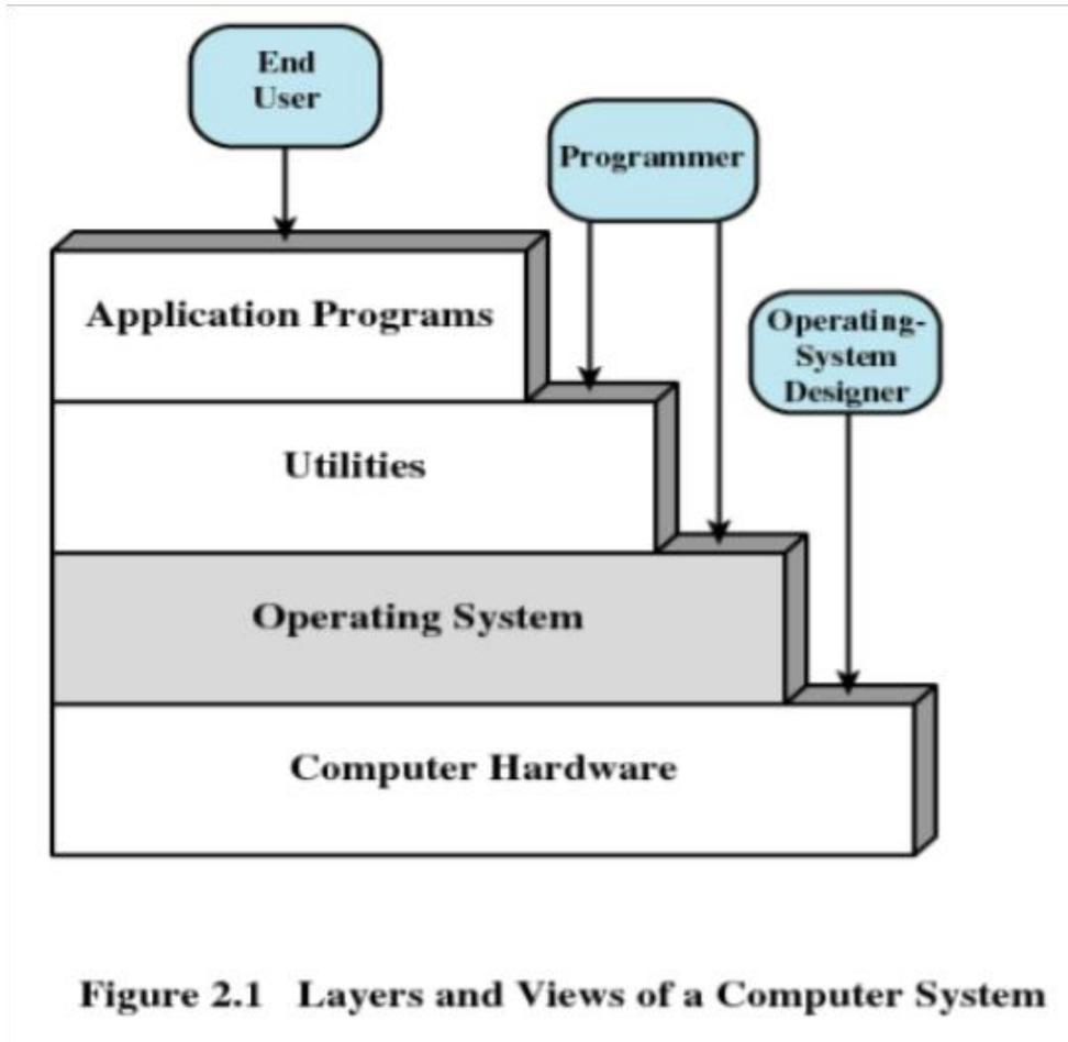
Figure 2.1 Layers and Views of a Computer System
